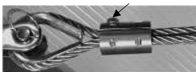
Picture 2 : Screw the nut to maintain the tension
