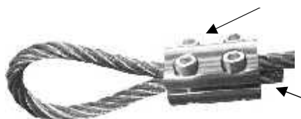
Picture 3 : Screws on the direction of the active strand
